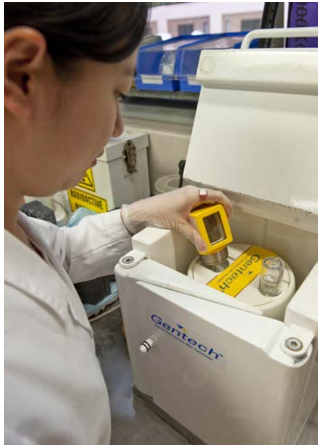
FIG. 9.9. Lead garage surrounding a ^{99}\text{Mo}/^{99\text{m}}\text{Tc} generator:
