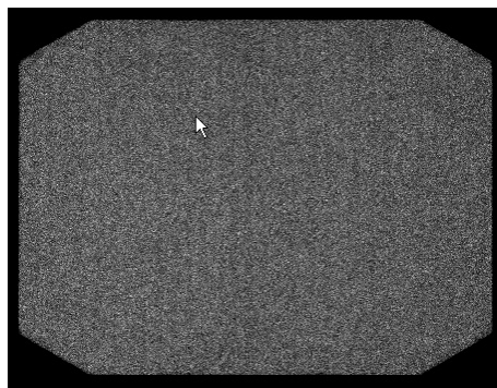
FIG. 11.6. Uniformity image of a defective foil collimator. The vertical stripes in the image result from non-uniform sensitivity of the collimator due to problems in the manufacturing process. The peppery texture is due to quantum noise and is visible because the grey level was expanded to demonstrate the non-uniformity artefacts.
