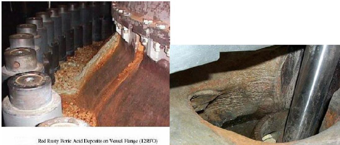
Rod Rusty Boric Acid Deposits on Vessel Flange (12RF0)
